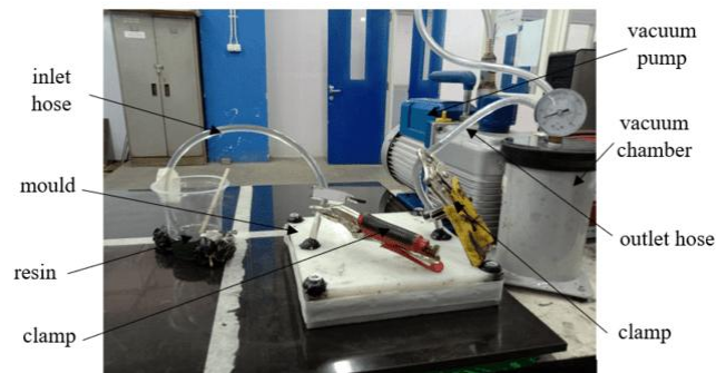
Figure 4 Vacuum Resin Infusion Process
